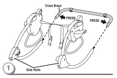
While pressing the tab on each end of the cross brace, insert the cross brace into the side rails, as shown. Make sure you hear a "snap" on each side.
